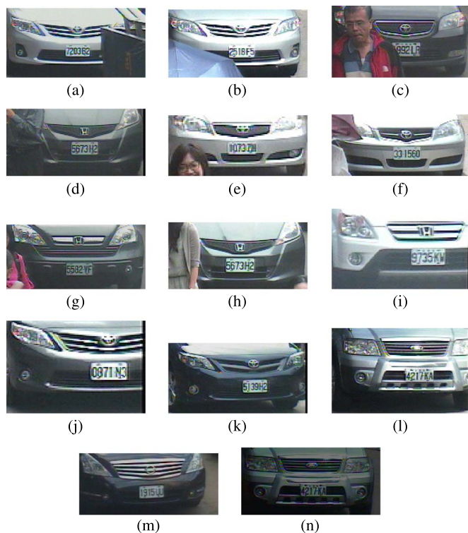
Fig. 17. Some challenging cases of vehicles under (a)–(h) occlusion, (i) and (j) partially out of the view of the camera, (k)–(m) nonfrontal views, or (m)–(n) under low lighting. The BoSURF-based VMMR approaches were successful in predicting the make–model class in the above cases.
